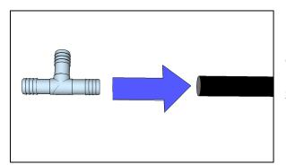
Barbed Fittings fit into vinyl tubing easily. Simply insert the barbed end into the vinyl tubing of desired length. Submerge the parts in water for easier push on connections.
